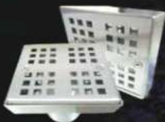
SKIRT ROOF DRAIN SS 304 - 100 X 100 BODY & SECURED GRATE 2" SIDE BOTTOM OUTLET Suitable for balconies & small open areas
